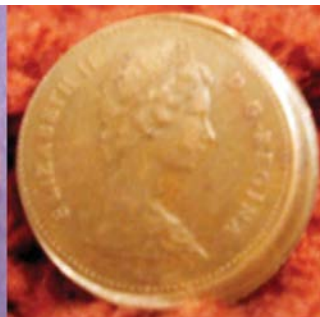
Figure 1. This coin is described as having been struck by a 'misaligned planchet.'
