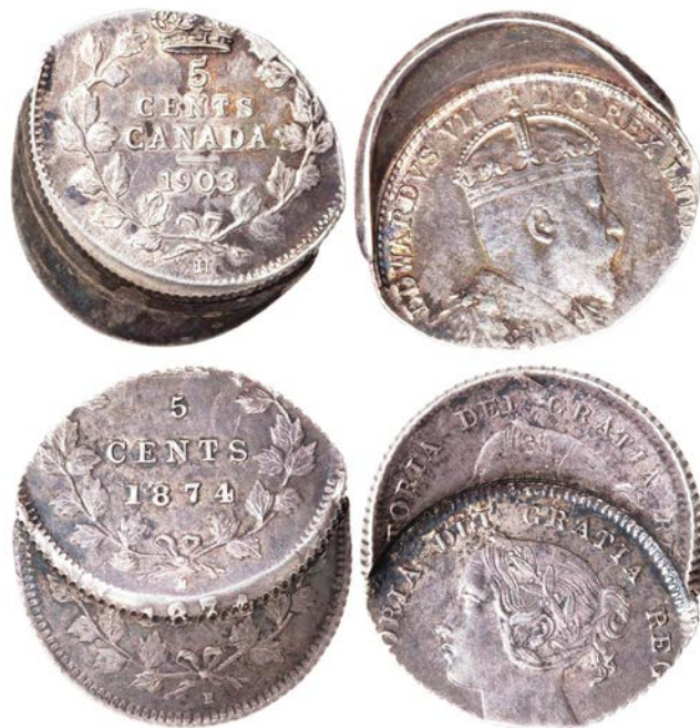
Figure 4. Because of the 'bend,' these two coins were struck with the 'wrong' die setup.
